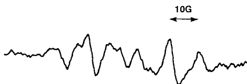
FIG. 3. ESR spectrum observed at 60°C in the ENMA/MAIB/benzene system: [\text{ENMA}] = 1.00 \text{ mol} \cdot \text{L}^{-1} ; [\text{MAIB}] = 1.00 \times 10^{-1} \text{ mol} \cdot \text{L}^{-1} .
